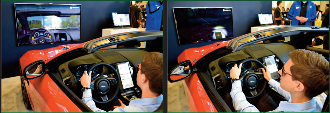
Using a dot on a screen, the Seeing Machines demonstrator at CES 2015 showed clearly how its technology can track a driver's line of sight - and that it works even if the driver is wearing sunglasses
