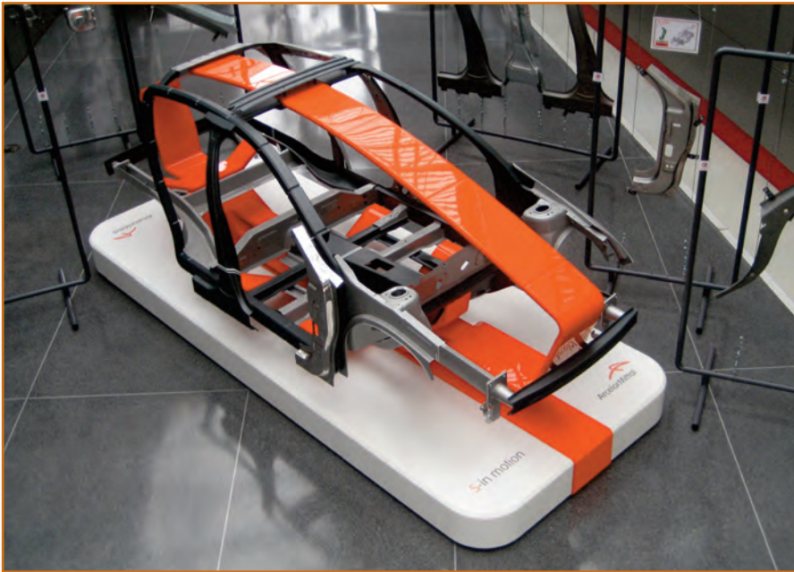
S-in motion demonstrator showing ArcelorMittal's automotive steel solutions
